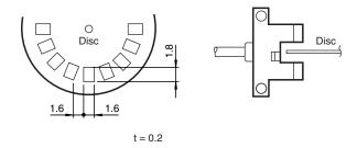
$\begin{tabular}{ll} \textbf{Response frequency}\\ \textbf{The response frequency is the value when the disc is rotated, see figure.} \end{tabular}$
